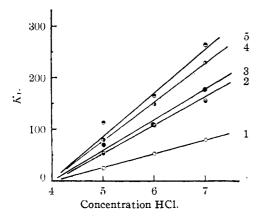
Fig. 3.—Relation between Boguski's constant and the conen. of hydrochloric acid used. (1) Cd + 0.79 at. % Au, 25°; (2) Cd + 0.79 at. % Au, 40°; (3) Cd + 0.48 at. % Pt, 25°; (4) Cd + 0.48 at. % Pt, 40°; (5) Cd + 0.98 at. % Pt, 25°.
