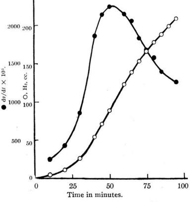
Fig. 2.—The solution rate of Cd + 0.98 at. % Pt in 6 N HCl, at 40°, without mechanical stirring. The upper curve shows the solution rate with time, the lower, the amount of hydrogen evolved in the same time.
